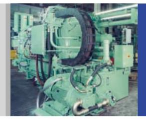
Pressure cast machine, pump with variable pump flow thanks to drive speed control
